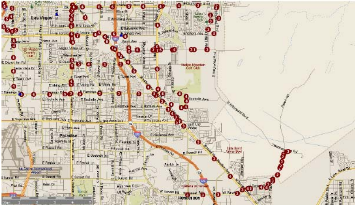
Figure 6-15. Observed Numeric CO Concentrations (ppm) During December 19 to 20 Evening/Night Period Concentrations illustrate the drainage flow. DAQM sites are shown in blue triangles.
